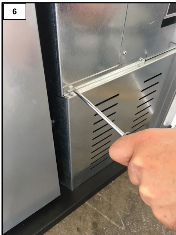
Remove the front guard (figures 6 and 7).
